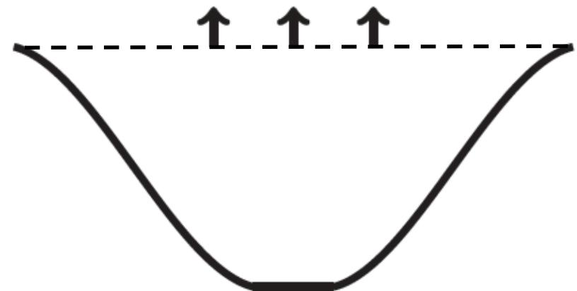
$$Q_{\text{exp}} = c_p \int_{t_r}^{t_s} \int_A \langle \bar{\rho} \rangle \langle \overline{\tilde{w}\tilde{\Theta}} \rangle \Big|_{z=h_c} dx dy dt$$
