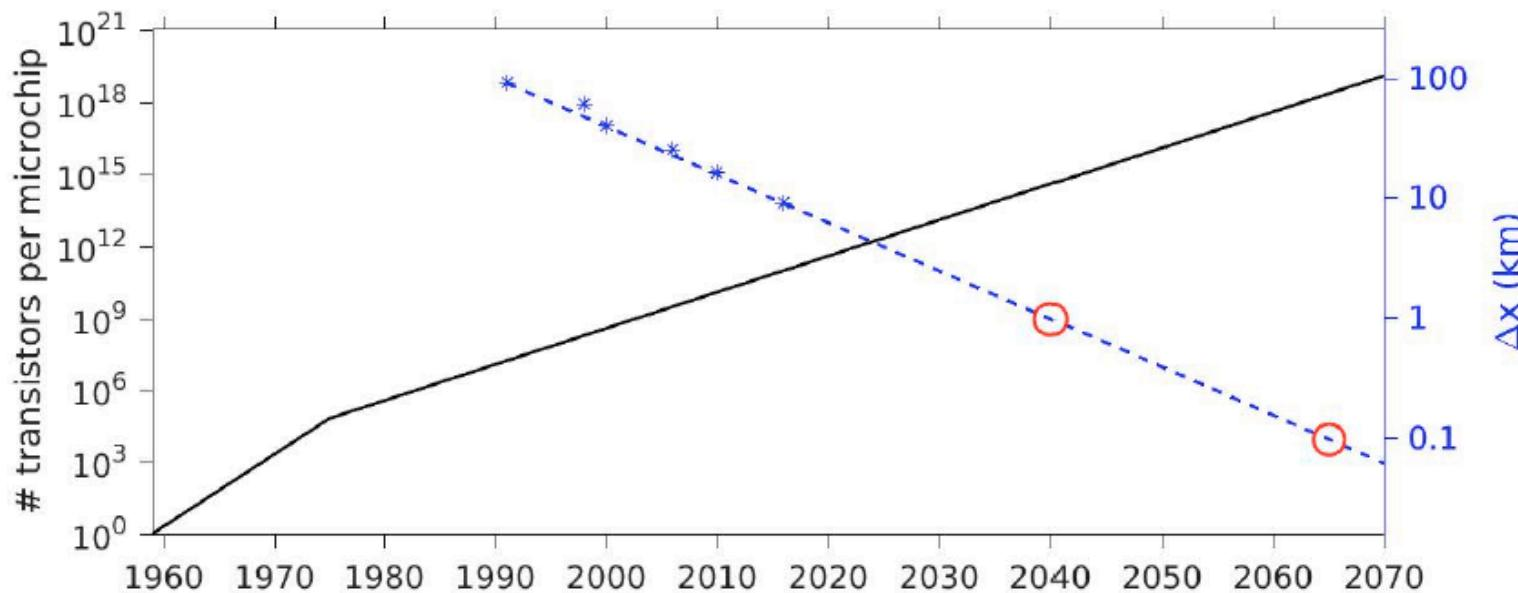
**Figure 6.** Number of transistors per microchip predicted by Moore's Law [139] (solid line, left scale) and horizontal grid spacing of the ECMWF IFS (asterisks, right scale). The dashed blue line is a fit that assumes dividing the grid spacing by two every 7.5 years and the red circles indicate the years when a grid spacing of 1 km and 100 m will be reached based on this fit.
